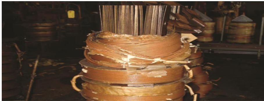
Fig. Inter turn faults...
